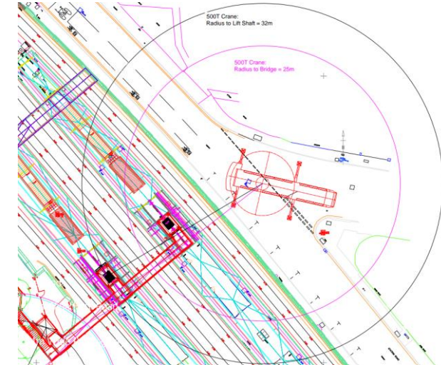
Crane positioned on Station Road for platform steelwork installation
