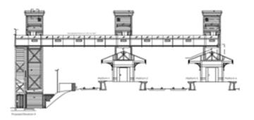
about the lift capacity and door width. Another drawback to the latest design is that passengers using the lifts will be required to use two lifts instead of one as originally intended and to walk 25m from the booking hall to the first lift. On the plus side, we now know that the three towers in the design will be clad with bricks matching the colour and banding of those in the present station structure.
